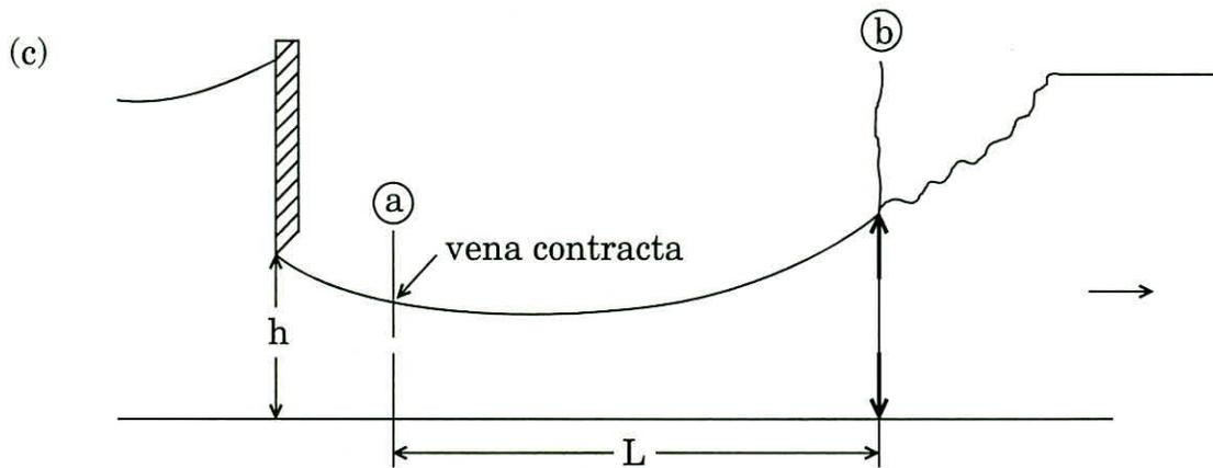
Consider a vertical sluice gate in a wide rectangular channel. The depth of flow at the vena contracta is 0.457 m for a flow rate of 4.646 m<sup>3</sup>/s per metre of width. The channel bed slope is 0.0003 and Manning's roughness factor is  $n = 0.020$ . The depth of flow at point b is 0.5 m.
