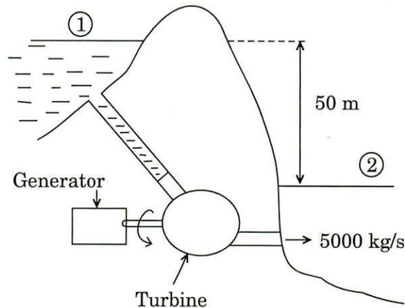
Density of water is  $1000 \text{ kg/m}^3$  and gravitational acceleration is  $9.81 \text{ m/s}^2$ .
