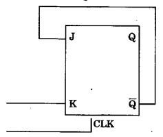
Assuming the flip-flop was initially cleared and then clocked for 6 pulses, the sequence at the Q output will be
