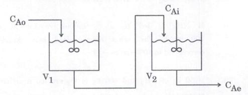
Comment on the values of the volume obtained for two CSTR's in series with that of the volume for one CSTR and volume required for a PFR.
